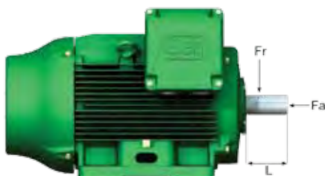
Figure 20 - Radial and axial thrust on motor shaft
