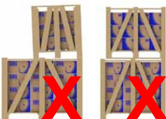
Figure 5.4 – Incorrect stacking
