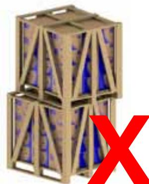
*Figure 5.2 – Incorrect stacking*
