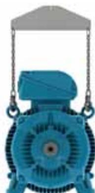
Figure 4.6 – Use of a spreader bar for lifting.
