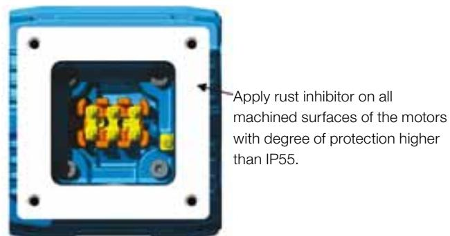
**Figure 8.2** - Machined surface of the terminal box of explosion-proof Motors.
